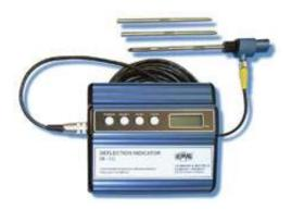
The LEMAG DI-5C electronic deflection indicator is the latest innovation in crankshaft deflection measurement. Originally the measurement was made by using a mechanical micrometer dial. This was time consuming, risky, unpleasant and dirty and a consequence these tasks were often avoided,
